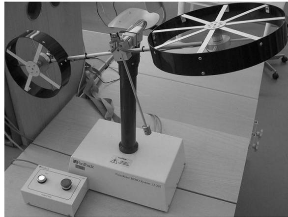
Fig 1: Twin rotor multiple input-multiple output system
