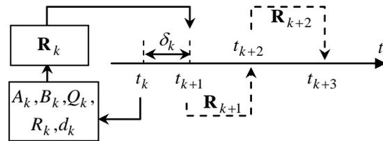
Fig 2: Receding horizon control with optimization
