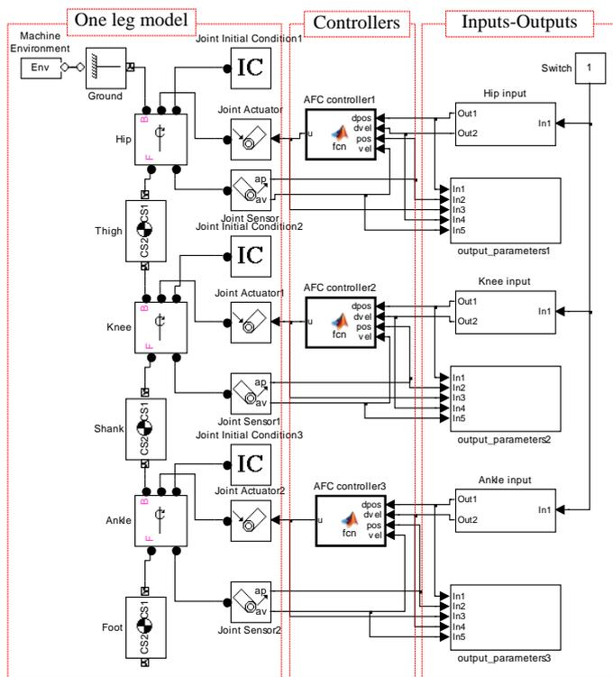
**Fig.11. Simulation model of 3 DOF exoskeleton system**
