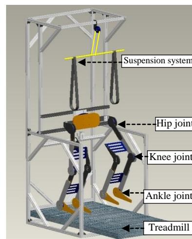
Fig.1. Structure of the exoskeleton
