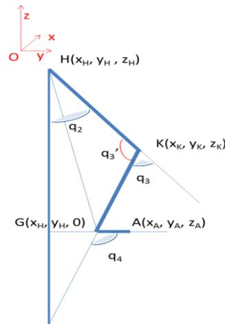
Fig.3. Geometric method for inverse kinematics calculations
