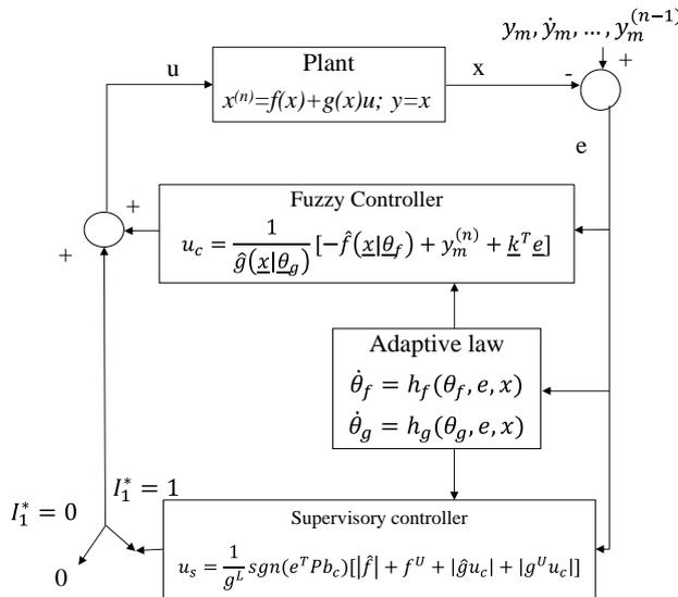
Fig.4. Block Diagram of an Adaptive Fuzzy Controller
