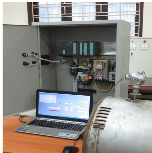
Fig 4: Temperature system implemented with PLC S7-300
