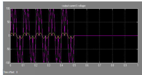
Waveform shows the output current & voltage, the input frequency is 2 times the output frequency
