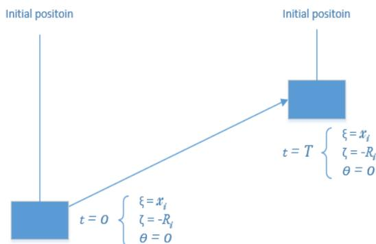
Fig.2. Load displacement in straight line crane
