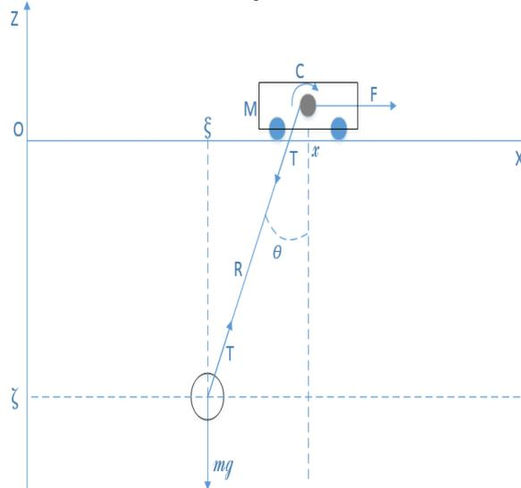
Fig.1. Two – dimensional overhead crane
