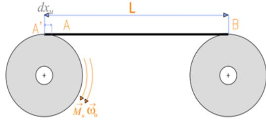
**Fig.4: The web transport system with deformation on unwinder web side**
