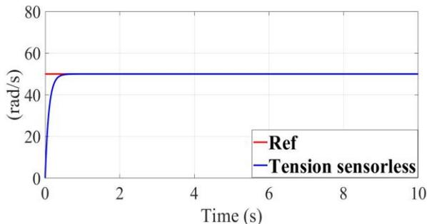
Fig.7: The angular velocity response with constant reference
