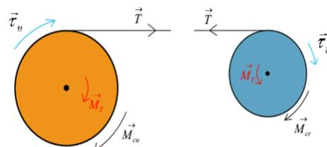
Fig.2: Unwinder and rewinder with torque and force
