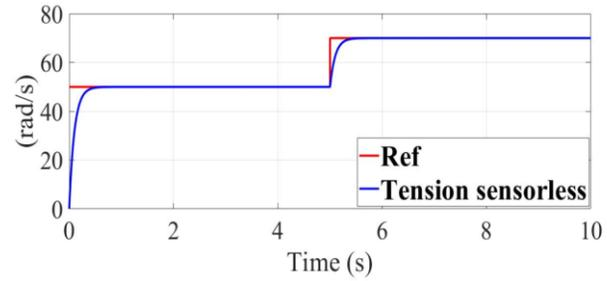
Fig.8: The angular velocity response with change reference
