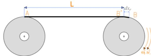
**Fig.5: The web transport system with deformation on rewriter web side.**
