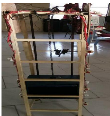
Figure3: Pictorial view of elevator design
