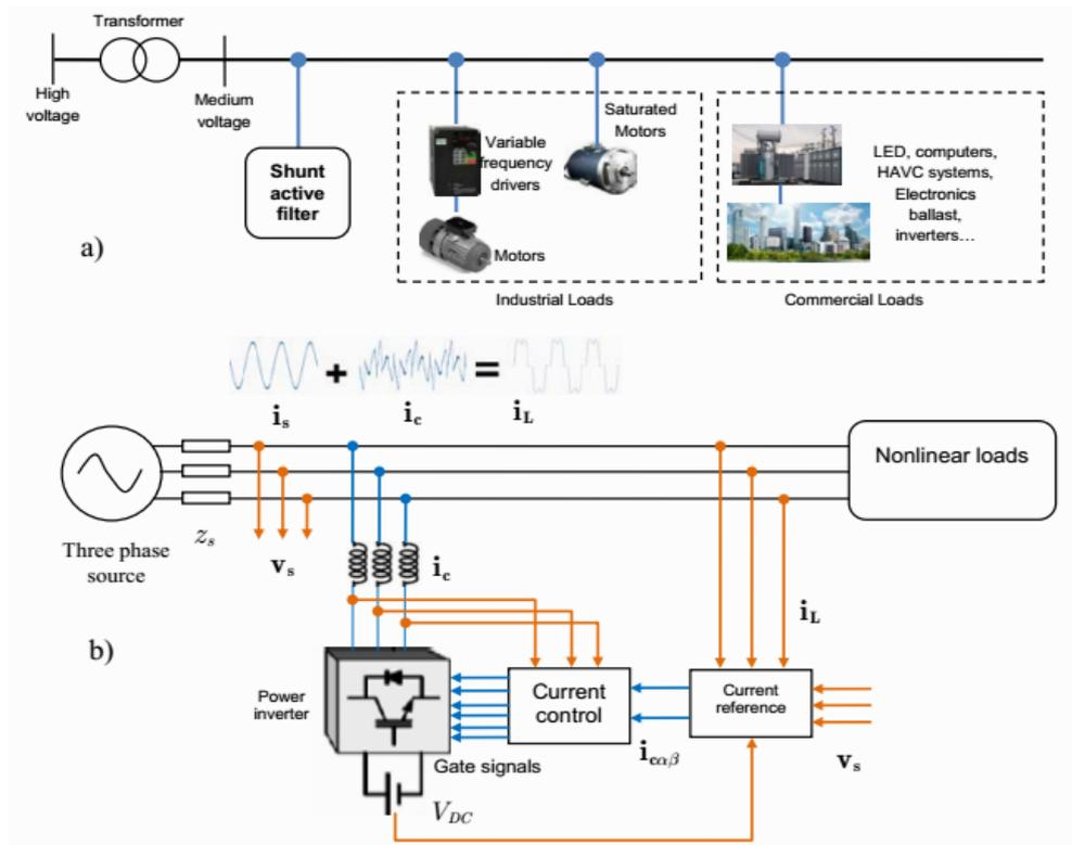
Fig 1: a) The position of SAF on the power system, b) The typical structure of SAF using the CCVSI
