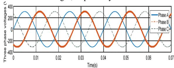
Fig 6. The 3 phase source voltages
