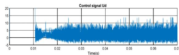
**Fig 14. The control voltage of SAF on the d frame**
