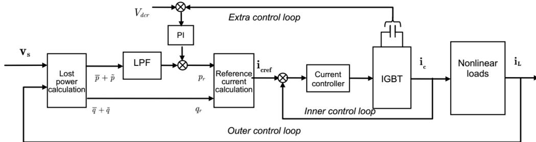
Fig 2: The structure of control loops of SAF
