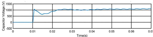
**Fig12. The varying of the voltage across capacitor of the SAF**
