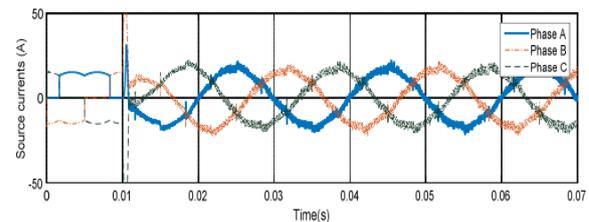
Fig 8. The source currents when using SAF
