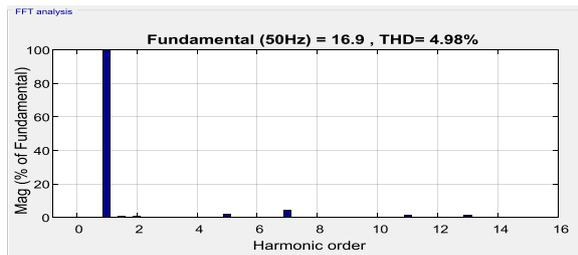
**Fig 11. The harmonic analysis of the source when using SAF**
