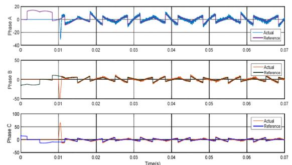
**Fig. 9. The compensation currents determined by the outer control loop and the real compensation currents made by inner loop to inject to the network**
