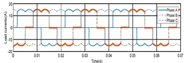
Fig 7. The load currents or source currents in the case not using SAF
