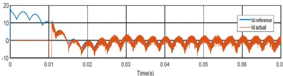
**Fig 13. The desired compensation currents and real currents on the d frame**
