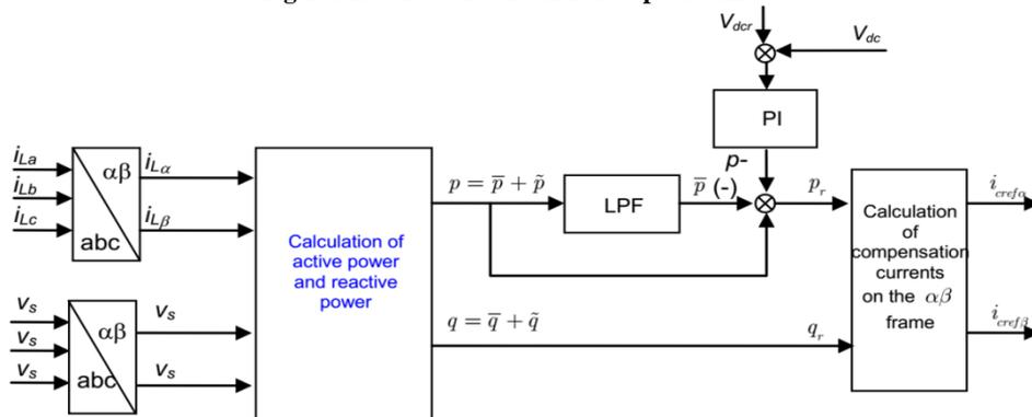
Fig 3: The structure of outer control loop
