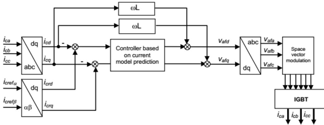
Fig 4. The control structure of SAF's inner loop based on current model prediction
