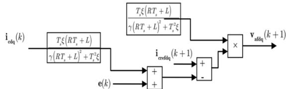
Fig5. The diagram for inner controller of SAF based on current predictive model
