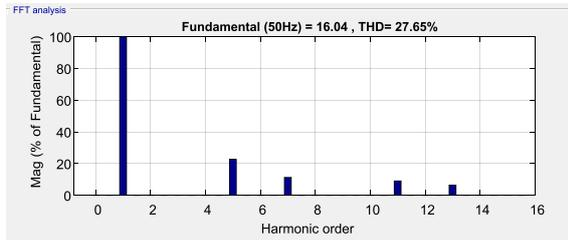
**Fig10. The harmonic analysis of the load currents**
