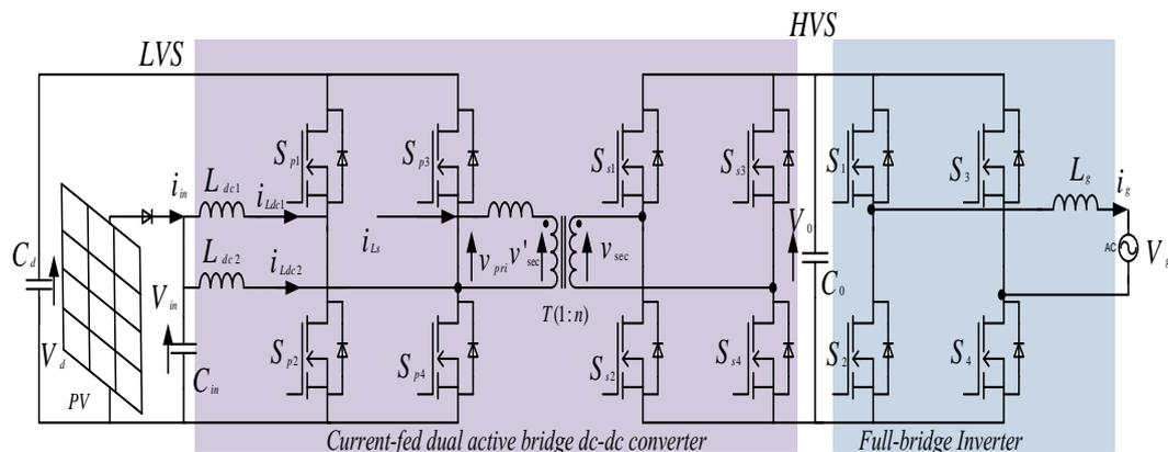
Fig.2 Proposed single phase grid connected PV system
