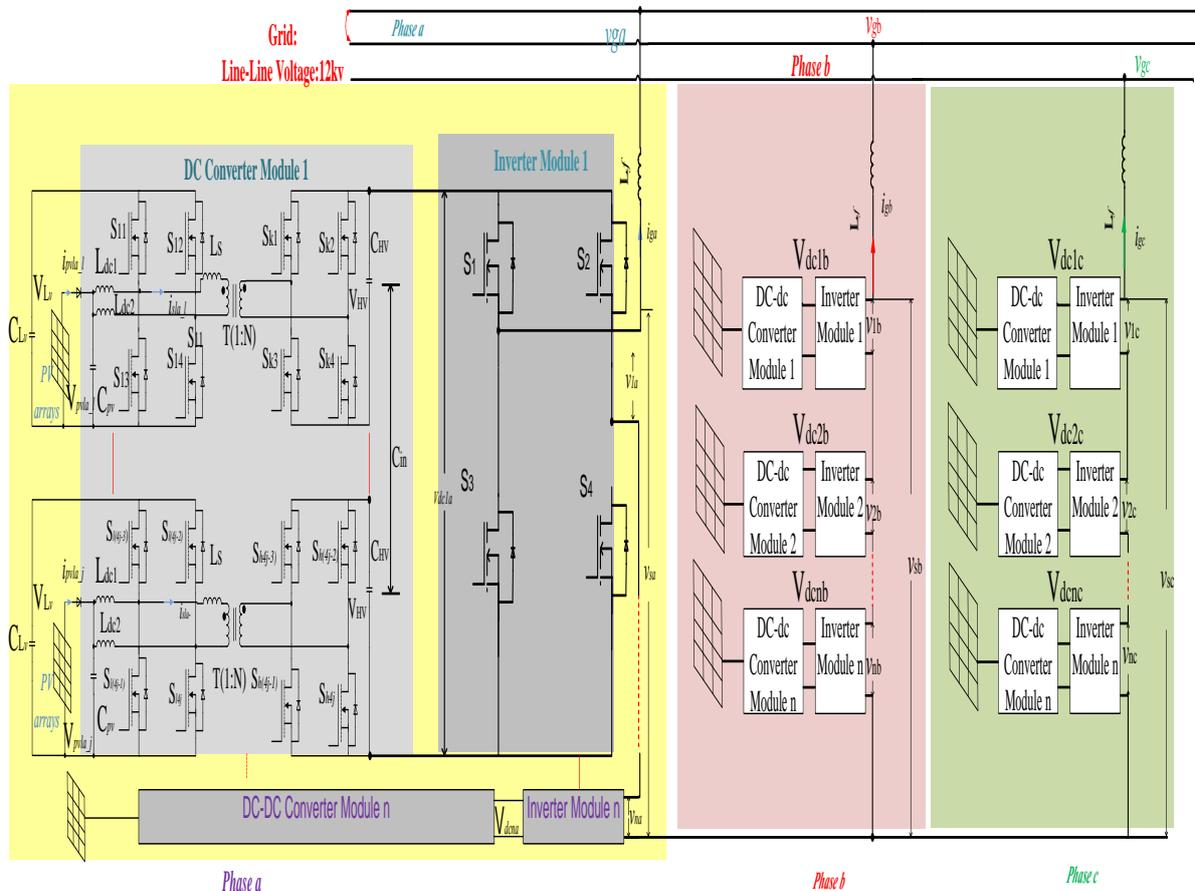
Fig.3 Proposed three phase grid connected cascaded PV system
