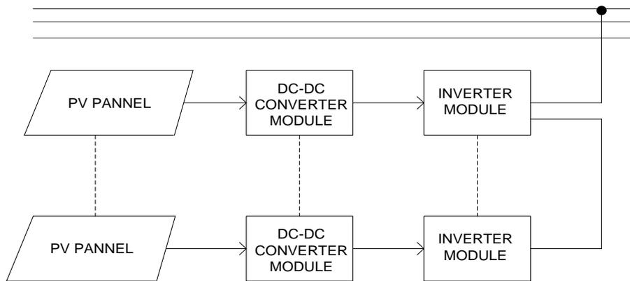
Fig.1 Block Diagram of cascaded PV system for one phase
