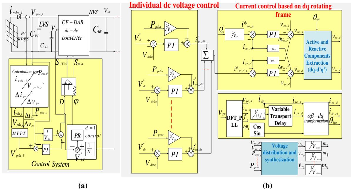
Fig.4 Control system of grid connected cascaded PV converters in phase a
