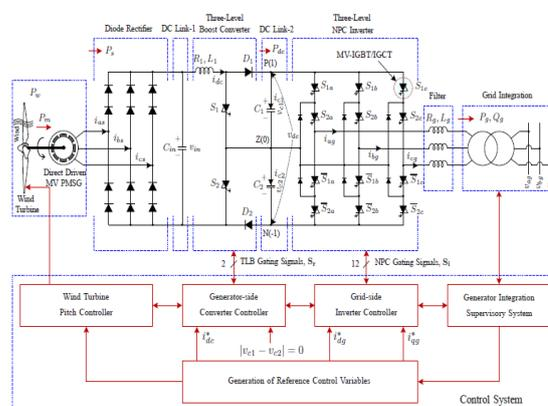
Fig 5. Configuration of three level boost converter and NPC inverter based MW-MV PMSG-WECS.
