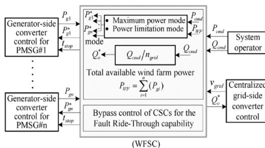
Fig 4. Block diagram of proposed wind farm.
