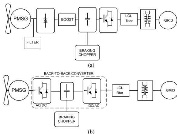
Fig. 11. Wind-turbine system. (a) Diode-bridge rectifier and boost converter. (b) Back-to-back converter.
