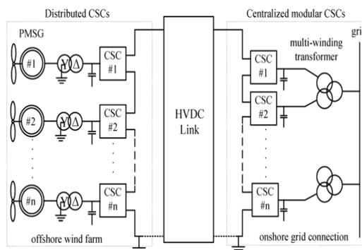
Fig 3. Proposed system configuration of cascaded CSC-based offshore wind farm
