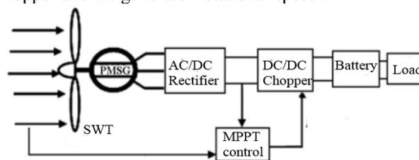
Fig 1. Schematic diagram of control system of a permanent magnet generator directly driven by wind turbine
