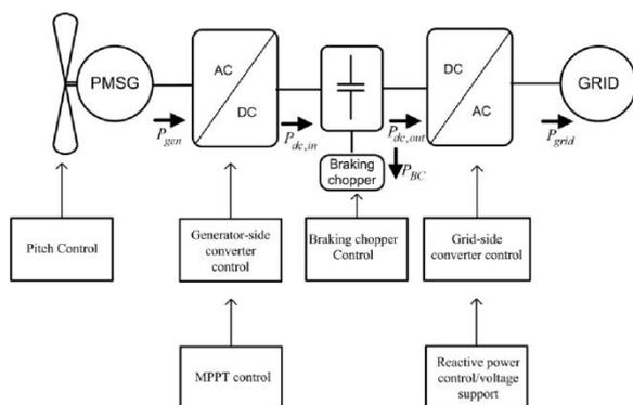
Fig 10. Control issues in PMSG-based small wind-turbine systems.
