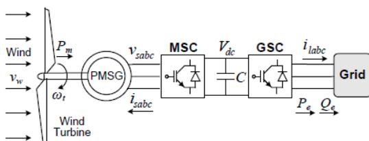
**Fig 6. Configuration of a direct-drive PMSG wind turbine.**
