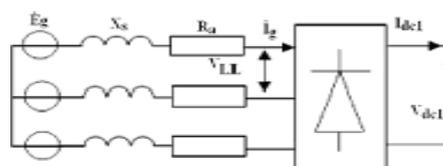
Fig 2. Connection diode rectifier circuits to the generator
