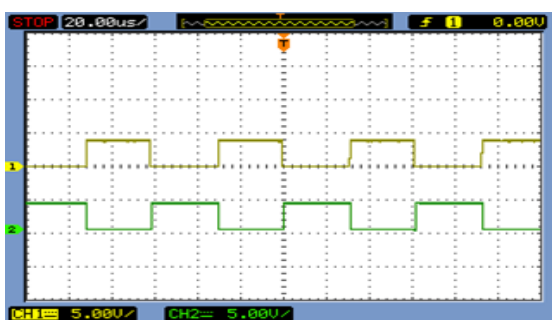
Fig 16: Switching pulse for converter switches
