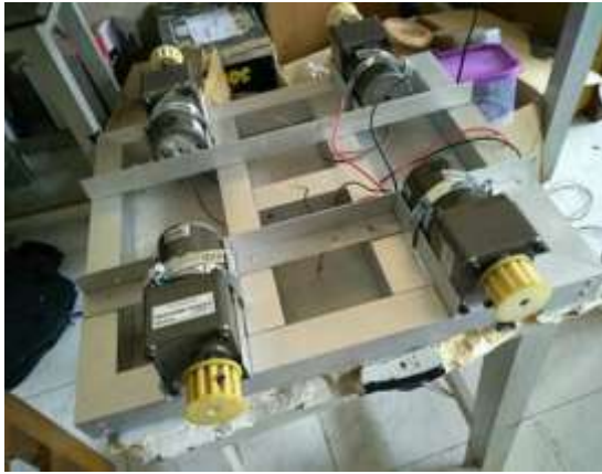
Fig 3: Chassis of farm-bot
