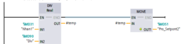
Figure 9: Program block for controlling PLC Client stations
