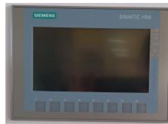
Figure 4: HMI screen KTP 700 Basic PN
