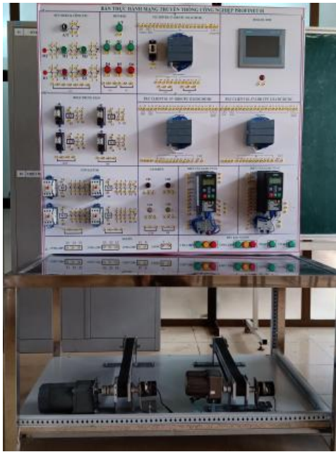
Figure 1: Device layout on Profinet network practice model
