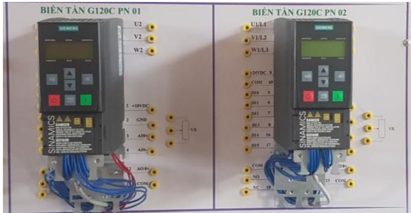
Figure 5: Model of G120C PN inverter
