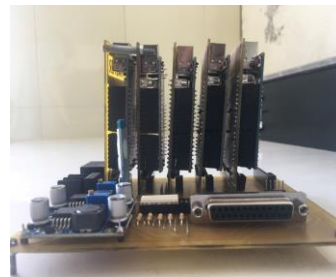
Figure 10: Control circuit images for the 5 degrees of freedom robot
