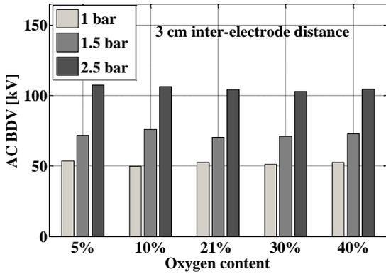
Fig. 2. AC breakdown voltages with 3 cm inter-electrode distance for different N<sub>2</sub>/O<sub>2</sub> gas mixtures and pressures
