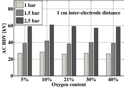
Fig. 1. AC breakdown voltages with 1 cm inter-electrode distance for different N<sub>2</sub>/O<sub>2</sub> gas mixtures and pressures.
