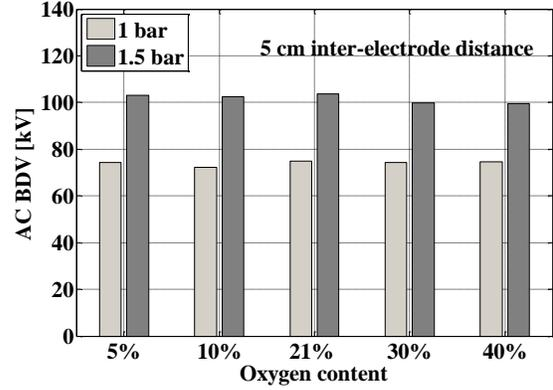
Fig. 3. AC breakdown voltages with 5 cm inter-electrode distance for different N<sub>2</sub>/O<sub>2</sub> gas mixtures and pressures.
