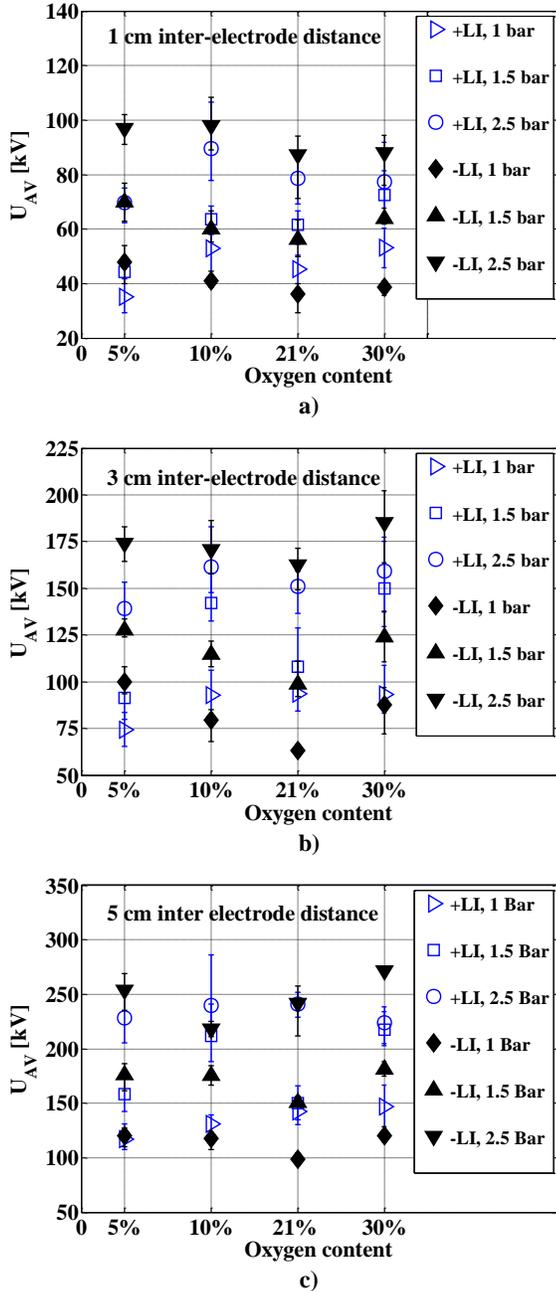
**Fig. 5. Impulse breakdown voltage in different N<sub>2</sub>/O<sub>2</sub> gas mixtures. Measured with 1 cm inter-electrode distance (a); measurement with 3 cm inter-electrode distance (b), and measurement with 5 cm inter-electrode distance (c). The error bars in the figures stand for the minimum and the maximum breakdown level during measurements.**
