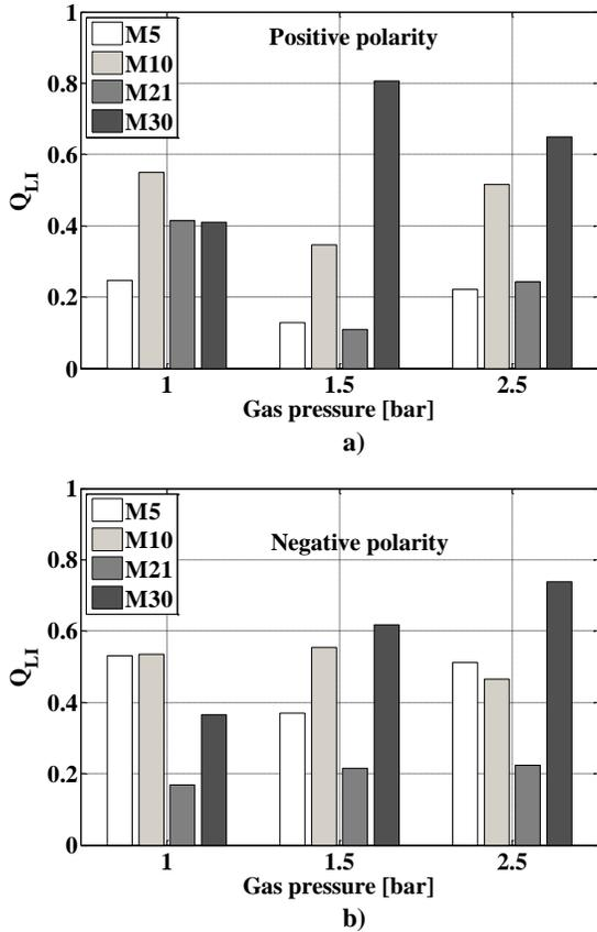
**Fig. 6. Quantity  $Q_{LI}$  against gas pressure for different  $N_2/O_2$  gas mixtures. Positive lightning impulse voltage (a), negative lightning impulse voltage (b)**
