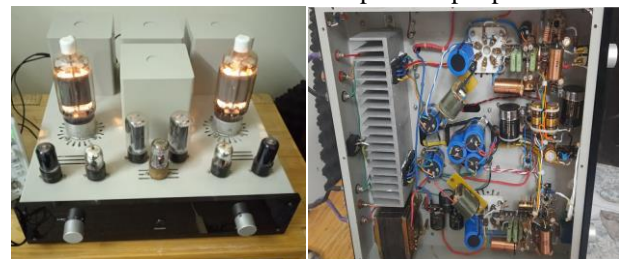
Fig 5: The outside image and the internal structure of the amplifier using an electron tube
