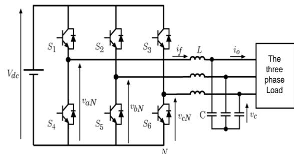
Fig 1: The three-phase inverter with output LC filter
