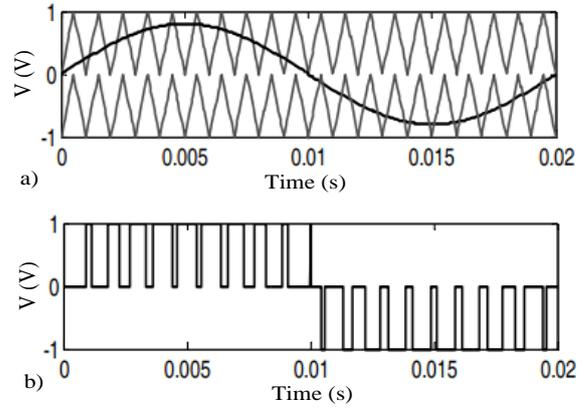
**Fig 5: a) Carrier waveform and modulation; b) the output voltage waveform**
