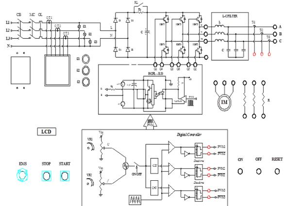
**Fig 9: The structure diagram of the reverse flow table with three-phase storage AC, motor control with load**
