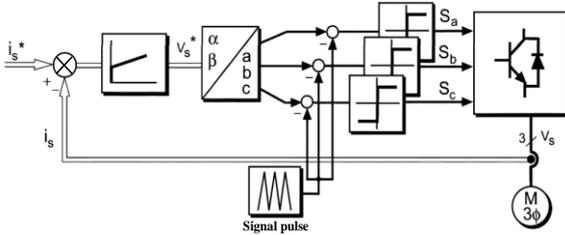
**Fig 4: The pulse width modulation current control**
