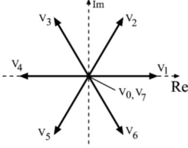
**Fig 2: The voltage vectors generated by the inverter**
