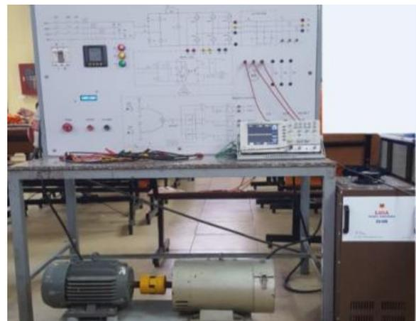
**Fig 10: Image of experimental structure of three-phase inverter flow in the laboratory**
