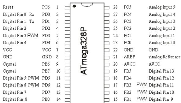
Figure 1.0: Arduino Pins Mapping
