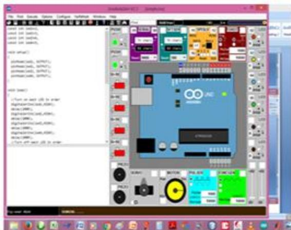
Figure 5.0 (b): Arduino Board-LCD Interfacing
