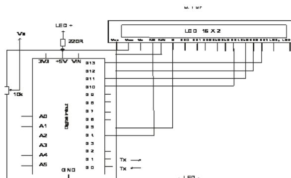
**Figure 3.0:** Arduino Board-LCD Interfacing
