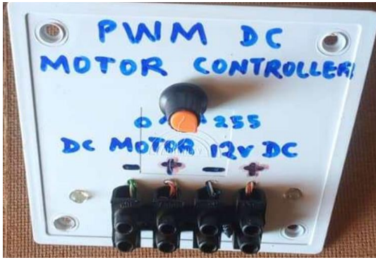
Fig. 6: Complete packaged PWM, DC motor controller system
