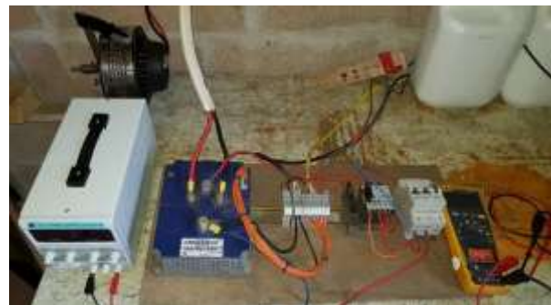
Fig. 7: 4PQM controller and LEM 170 DC Motor testing
