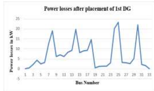
Fig. 5: active power losses after 1 st DG placement The optimal location obtained for placement of 2 nd DG unit is at 30 th bus with PSI value. After placement of DG the system loss reduced to 136.4704kW from 178.00kW as shown in Fig. 6.
