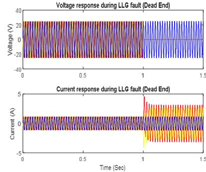
Fig 17: Voltage and Current waveform during L-L-G fault at Section-4.
