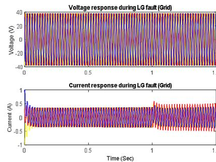
Fig 12: Voltage and Current waveform during L-G fault at Grid
