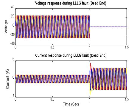
Fig 23: Voltage and Current waveform during L-L-L-G fault at Section-4.
