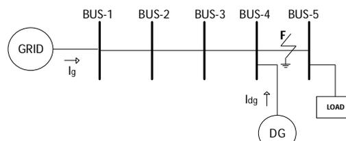
Fig 2: 5-Bus radial distribution system with DG
