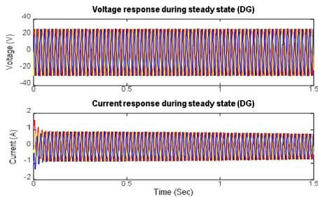
Fig 10: Voltage and Current waveform without fault at DG
