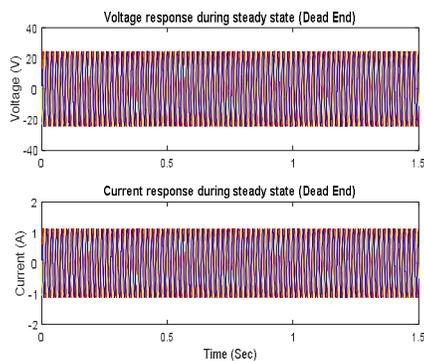
Fig 11: Voltage and Current waveform without fault at Section-4
