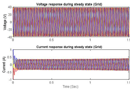
Fig 9: Voltage and Current waveform without fault at Grid
