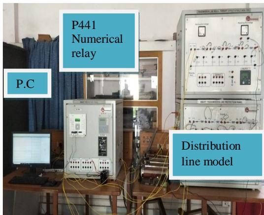
Fig 24: Practical Implementation in P441 Numerical Relay.
