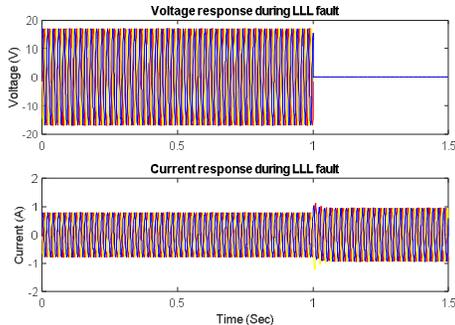
Fig 6: Voltage and Current waveform during Line-Line-Line Fault.
