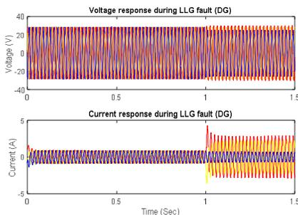
Fig 16: Voltage and Current waveform during L-L-G fault at DG
