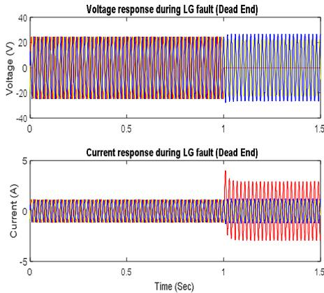
Fig 14: Voltage and Current waveform during L-G fault at Section-4.
