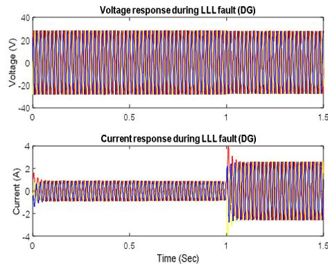
Fig 19: Voltage and Current waveform during L-L-L fault at DG
