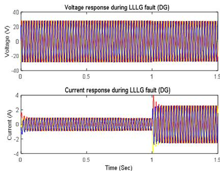
Fig 22: Voltage and Current waveform during L-L-L-G fault at DG
