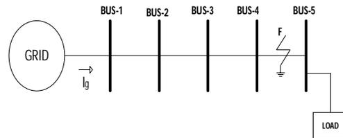
Fig 1: 5-Bus radial distribution system without DG
