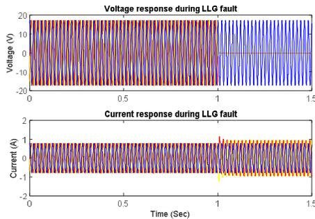
Fig 5: Voltage and Current waveform during Line-Line-Ground Fault.
