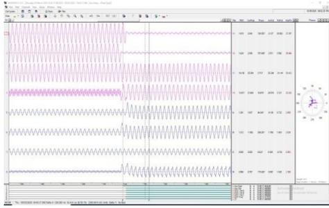
Fig 27: Voltage and Current waveforms during L-L-G fault
