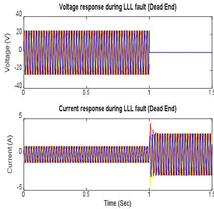
Fig 20: Voltage and Current waveform during L-L-L fault at Section-4.
