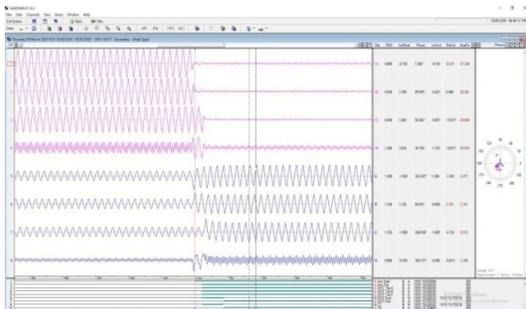
Fig 29: Voltage and Current waveforms during L-L-L-G fault
