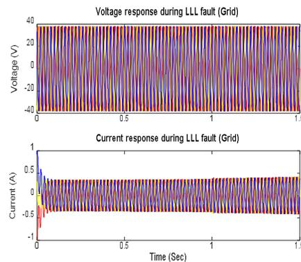
Fig 18: Voltage and Current waveform during L-L-L fault at Grid
