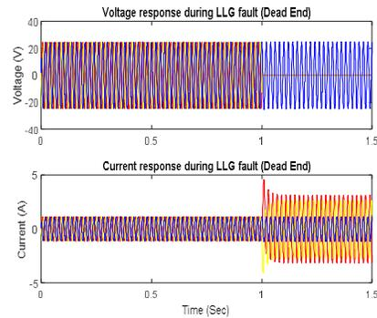
Fig 17: Voltage and Current waveform during L-L-G fault at Section-4.
