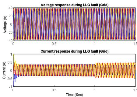
Fig 15: Voltage and Current waveform during L-L-G fault at Grid
