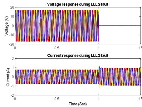
Fig 7: Voltage and Current waveform Line-Line-Line-Ground Fault.
