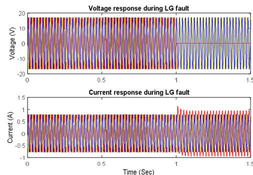
Fig 4: Voltage and Current waveform during Line-Ground Fault.
