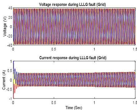
Fig 21: Voltage and Current waveform during L-L-L-G fault at Grid
