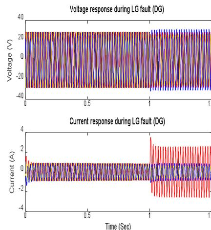
Fig 13: Voltage and Current waveform during L-G fault at DG
