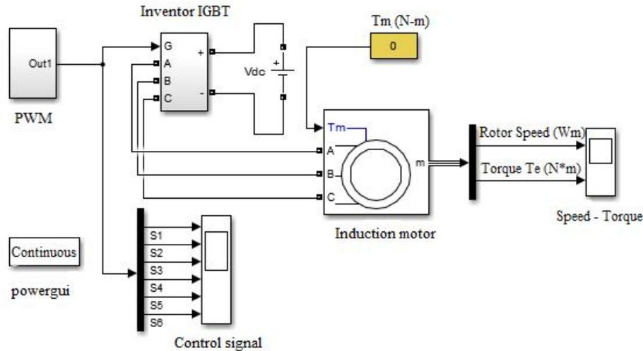
Figure 5: A simulation model of 3-phase asynchronous motor control on Matlab Simulink
