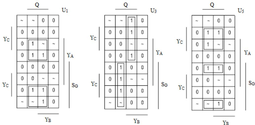
Figure 4: Karnaugh maps for logic functions U<sub>5</sub>, U<sub>3</sub>, U<sub>1</sub>
