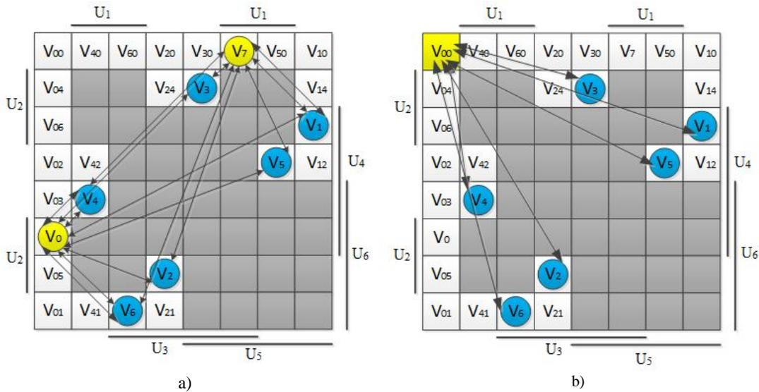
Figure 2: Karnaugh Maps asymmetric 180° switching a) with braking modes V<sub>0</sub>, V<sub>7</sub>; b) with braking mode V<sub>00</sub>
