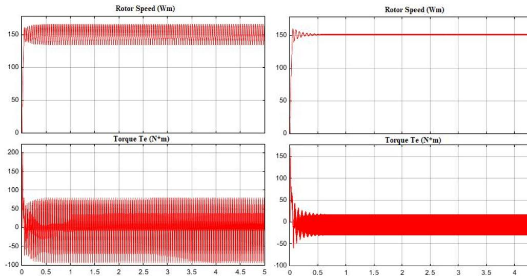
Figure 8: Speed and Torque Motor form when changing pulse-modulation frequency Q alternatively 6 and 12 times voltage pulse frequency corresponding to figures a and b
