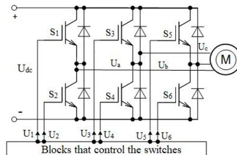
Figure 1: Three-phase inverter circuit diagram
