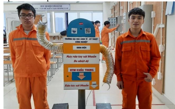
Fig. 1 The Body Thermal Measuring, Washing Hand Automatically Without Touching, And Giving Free Face Mask For Epidemic Prevention
