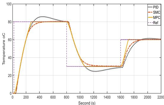
Fig. 8 Temperature control at different set-points
