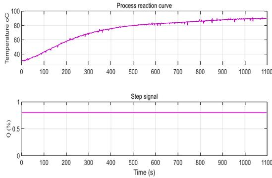
Fig. 3 Step response of the water tank
