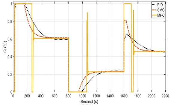
Fig. 9 Temperature control with input constraints
