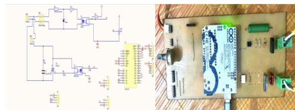
Fig. 2 The phase-angle control circuit
