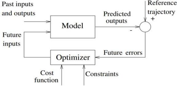
**Fig. 5 Basic structure of MPC**
