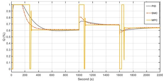
Fig. 7 The controller outlets with input constraints
