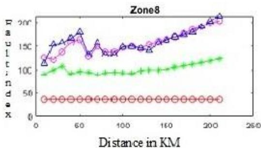
Fig. 45 LLL varying fault on zone-8 using coif1
