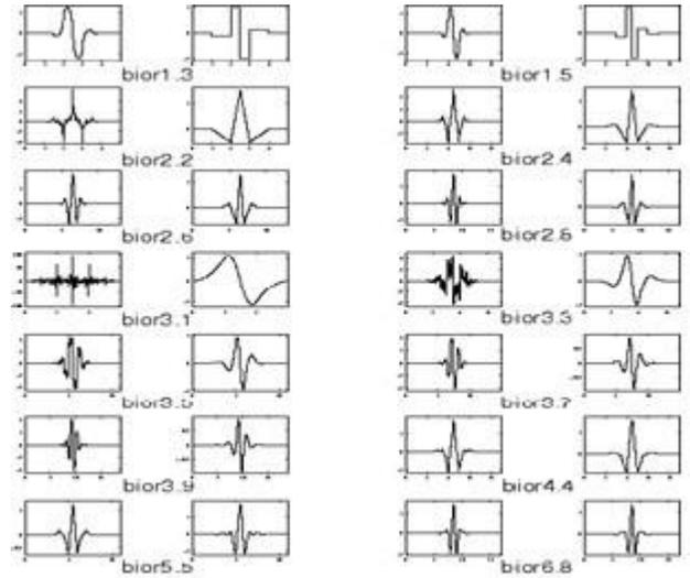
**Fig. 1 Types of biorthogonal wavelet**
