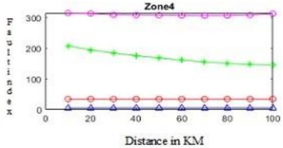
Fig. 23 LLL fault on zone-4 using coif1
