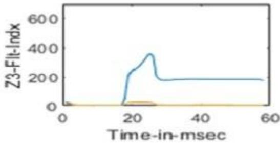
Fig. 7 L-G fault on zone-3 using morphing
