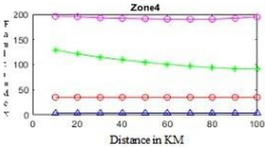
Fig. 20 LL-G varying fault on zone-4 using bior2.2
