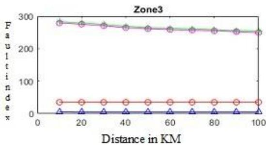
Fig. 16 L-L-L fault variation on zone-3 using coif1
