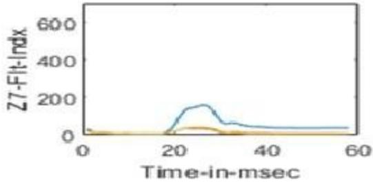
Fig. 26 L-G fault on zone-7 using ciof1
