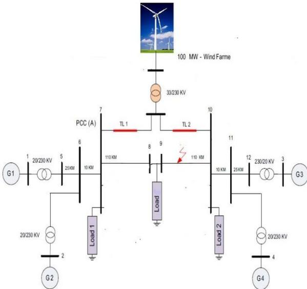
**Fig. 4 Single line diagram of the proposed system**
