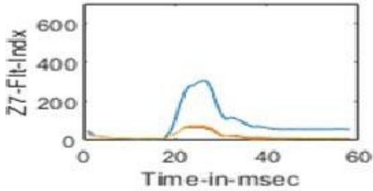
Fig. 27 L-G fault on zone-7 using morphing
