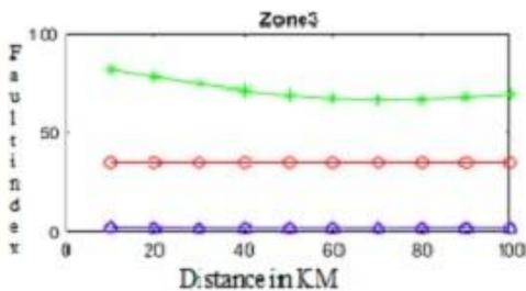
Fig. 8 L-G fault variation on zone-3 using bior2.2
