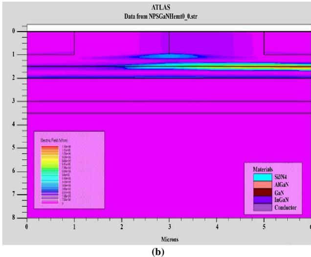
Fig. 7 Distribution of electric field around the gate electrode (a) without and (b) with a GFP
