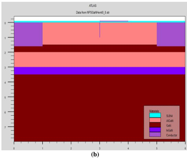
Fig. 4 Simulated structure of normally-off DH-HEMT a) with field plate and b) without field plate
