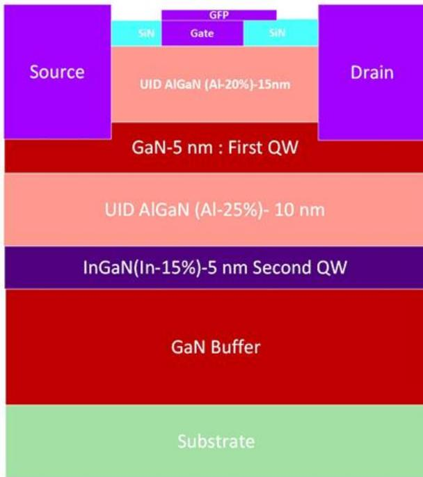
Fig. 1 Double quantum well EMODE structure with GFP and SiN passivation layer
