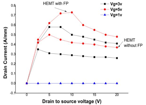
Fig. 5 HEMT with a gate field plate and typical HEMT output characteristics
