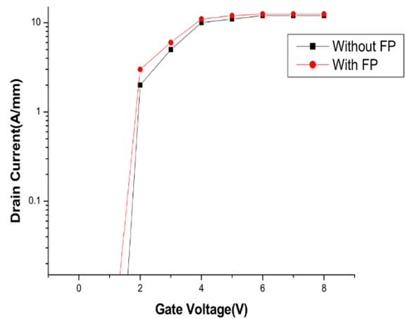
Fig. 6 Transfer characteristics of HEMT with a GFP and a regular HEMT
