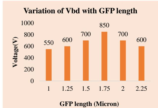
Fig. 9 Variation of breakdown voltage with the increasing length of GFP
