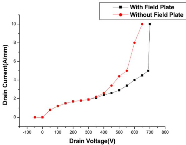
Fig 8. Breakdown characteristics of the device with and without field plate
