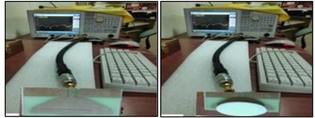
Fig. 12 Testing fabricated antenna in VNA
