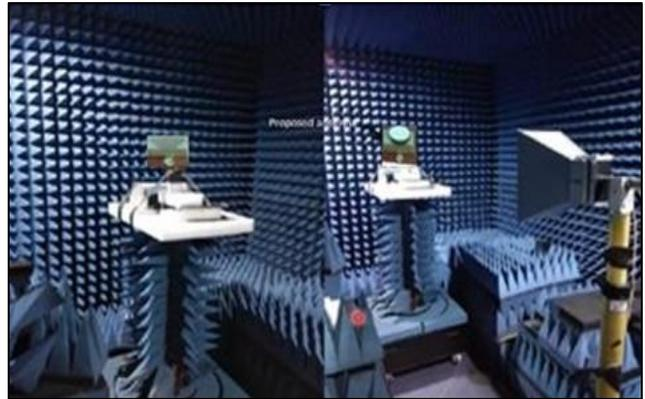
Fig. 13 Testing antenna in Anechoic Chamber
