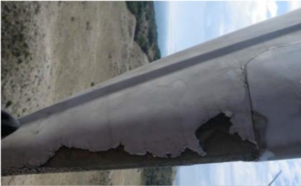
Fig. 13 Blade damage caused by erosion process
