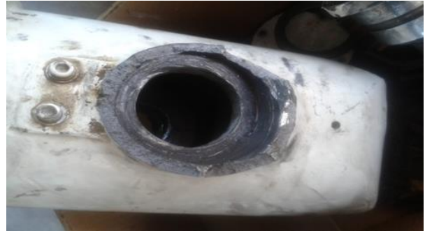
Fig. 3 Damage in the rotary part of a 2-kW wind turbine
