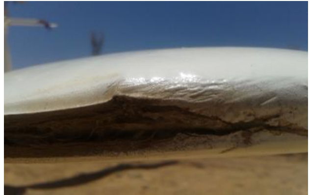
Fig. 11 Sign of blade ageing due to increase in temperature
