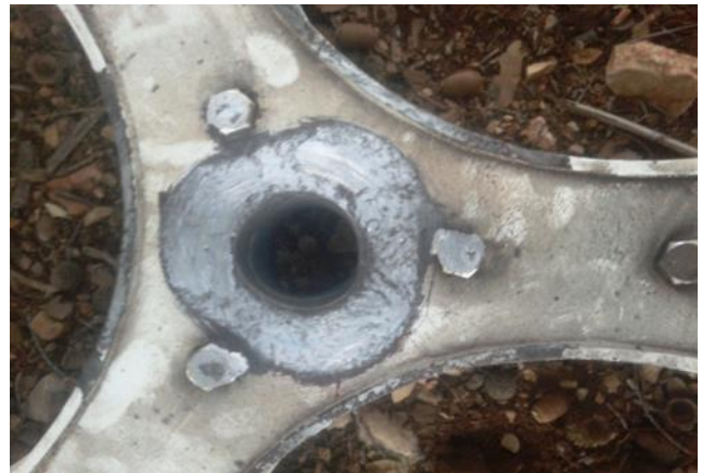
Fig. 10 Failure of the metallic bracket holding the blades
