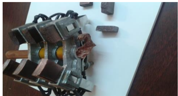
Fig. 6 Damage in the shaft, holding the brushing system
