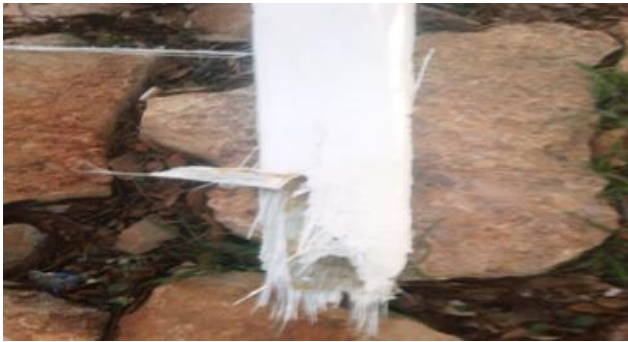
Fig. 8 Mechanical failure in the middle of the turbine blade
