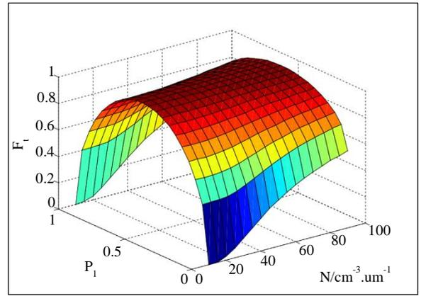
**Fig. 3 The relationship between the average fidelity of the depolarization channel and the probability of source characters and droplet concentration**
