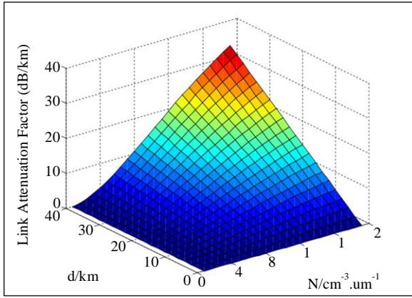
**Fig. 2 Relationship between link attenuation and transmission distance and droplet concentration**
