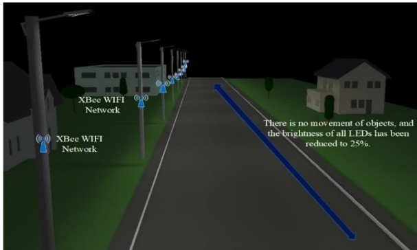
Fig. 6 XBee-based smart street lighting simulation during no object movement (25% brightness)
