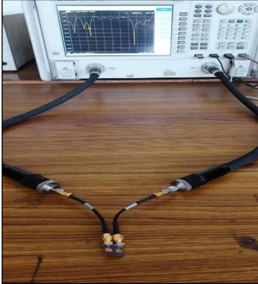
Fig. 21 Measurement of S-parameter of fabricated 2x2 MIMO
