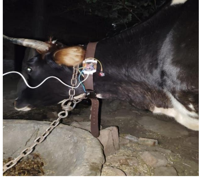
Fig. 5 Real-time execution of intelligent collar device
