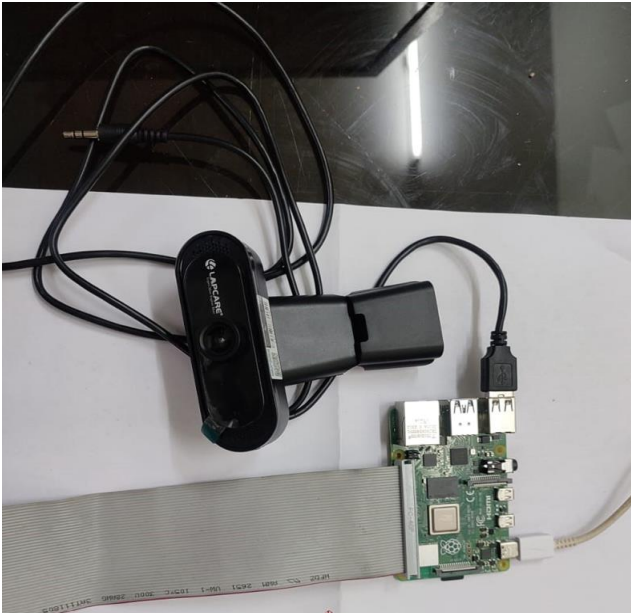
Fig. 2 Vision apparatus for observing the health of livestock
