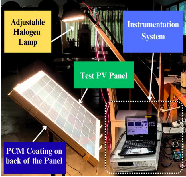
Fig. 2 Experimental setup: PV panel with adjustable Halogen lamp
