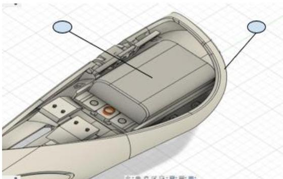
Fig. 5 Battery compartment
