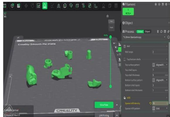
Fig. 7 The slicing process of prosthetic arm components, with the STL files prepared for 3D printing on a smooth PEI plate (Creality K1 MAX software).
