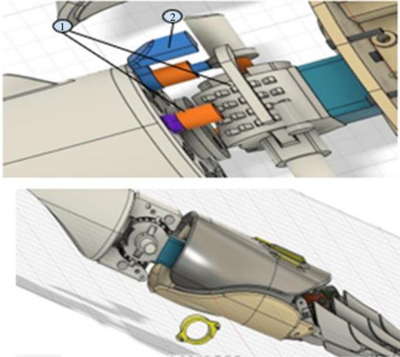
Fig. 4 Wrist mechanism, top view and side view
