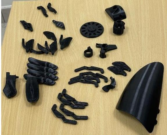
Fig. 8 3D-printed components of the prosthetic arm, fabricated by executing G-code instructions layer by layer, resulting in precise and high-quality parts that meet the design specifications.
