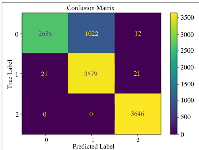
Fig. 15 Confusion matrix for classifying gripping (0), pinching (1), and twisting (2)
