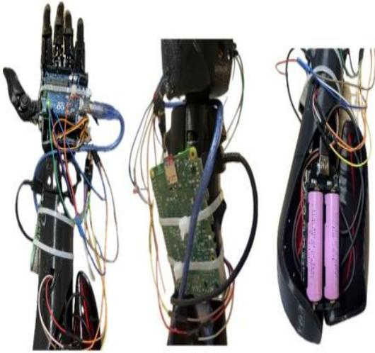
Fig. 11 The internal electrical configuration of the prosthetic arm.
