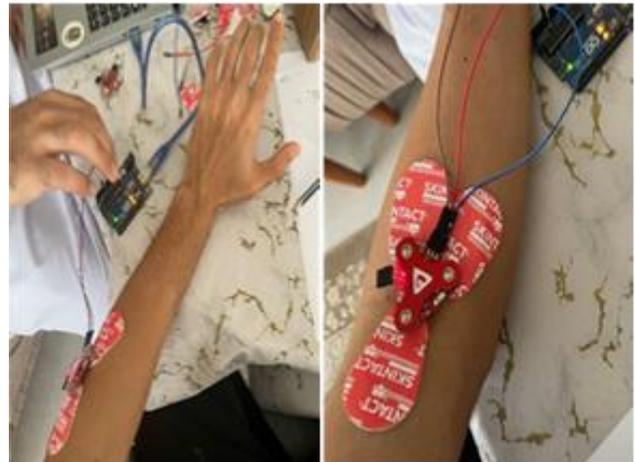
**Fig. 12** The setup used to record muscle activity during hand gestures. In the left image, electrodes are placed on the forearm to capture muscle signals while the subject gestures. The right image shows electrodes placed in a different muscle group.
