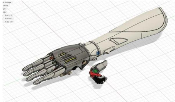
Fig. 6 The overall design of the prosthetic arm (fusion 360)
