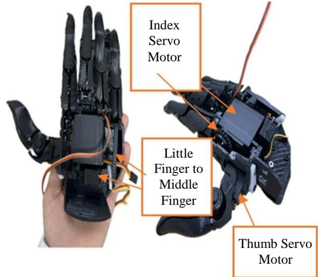
Fig. 10 Hardware integration of the prosthetic hand
