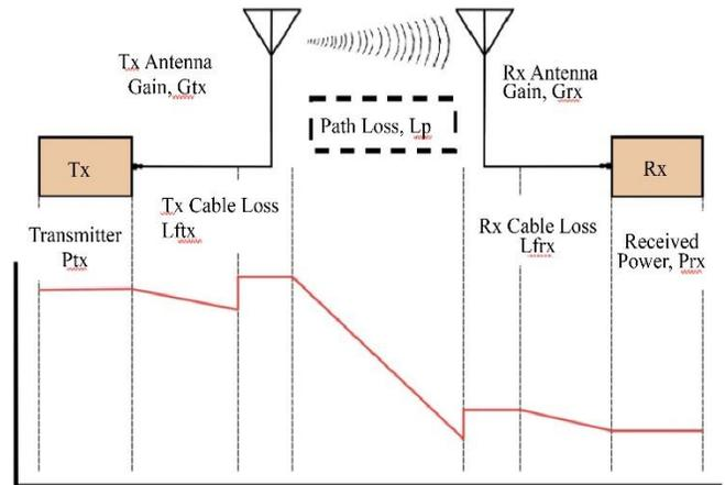
Fig. 4 A practical and simplified link budget design based on models for path loss
