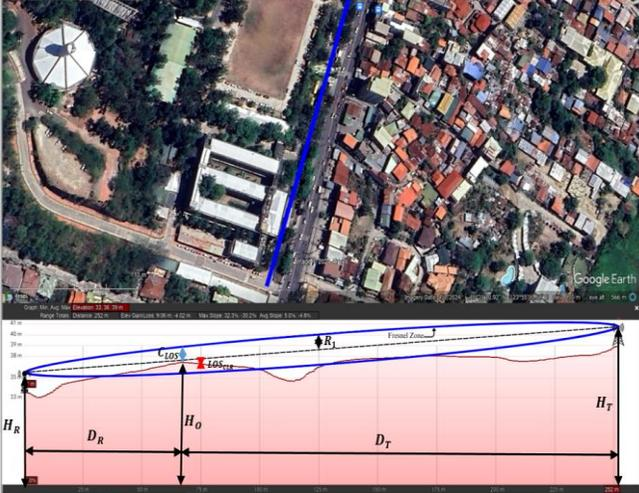
Fig. 6 Site 1 path profile traversing uneven terrain with obstruction at 1<sup>st</sup> Fresnel zone
