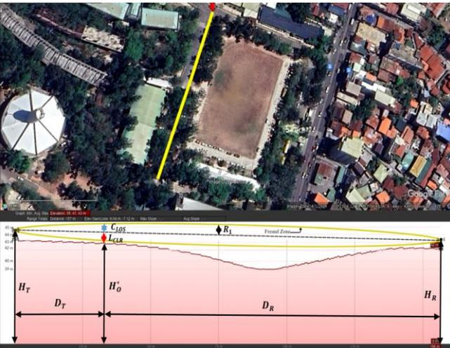
Fig. 7 Site 2 path profile traversing uneven terrain without obstruction at 1<sup>st</sup> Fresnel zone
