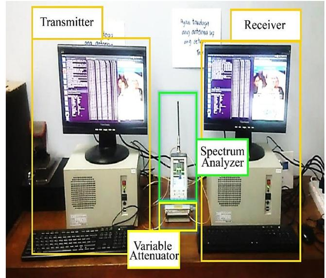
Fig. 1 IEEE 802.11af prototype developed by NICT used as AP and STA
