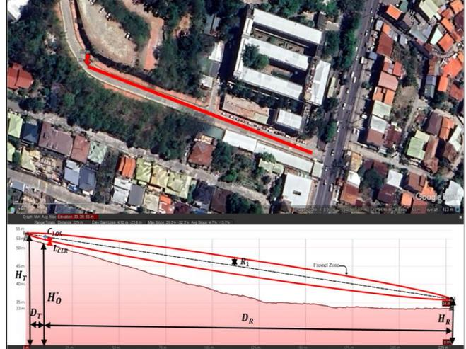
Fig. 8 Site 3 path profile traversing uneven terrain without obstruction at 1<sup>st</sup> Fresnel zone
