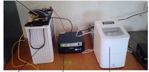
Fig. 9 Testing of ice cube machine with battery and inverter
