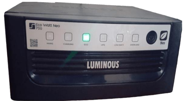
Fig. 6 Solar Charge Inverter (12V DC/230V AC, 1000 AC 50 Hz, 2000 watt)
