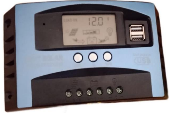
Fig. 4 MPPT 24/12-volt, 40 Amp solar charge controller
