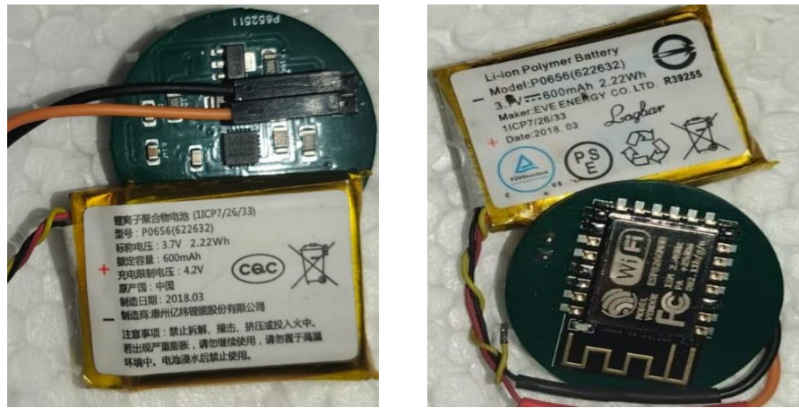
Fig. 4 Real-time Data Acquisition System (DAS)
