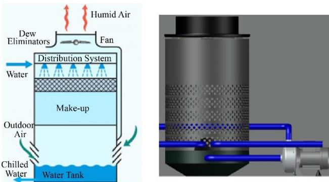
Fig. 12 Operation of cooling turrets
