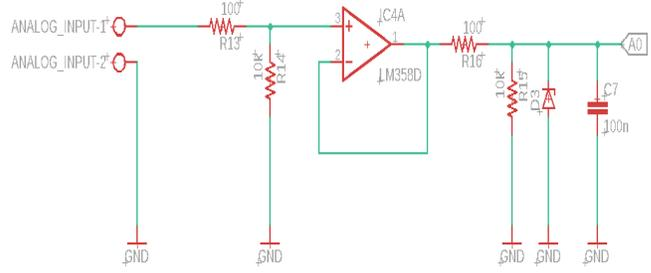
Fig. 5 0-10VDC to 0-5VDC input signal conditioning
