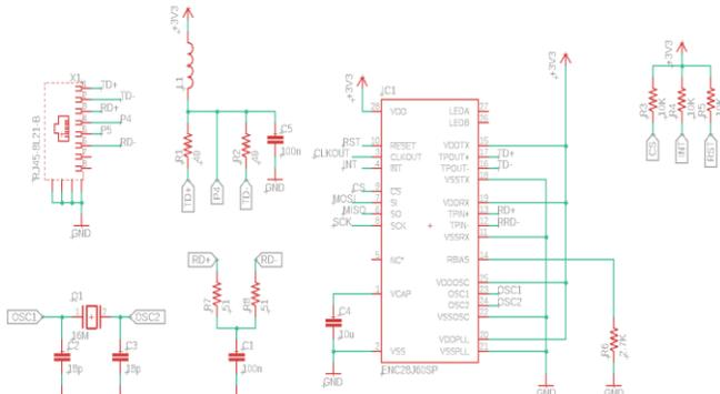
Fig. 3 MODBUS communication with ENC28J26
