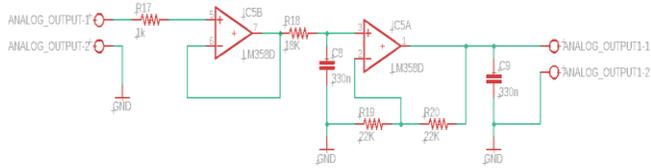
Fig. 6 0-5VDC PWM to 0-10VDC output signal conditioning
