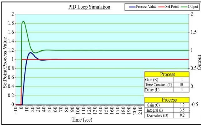
Fig. 11 Variable controlled with PID tuning
