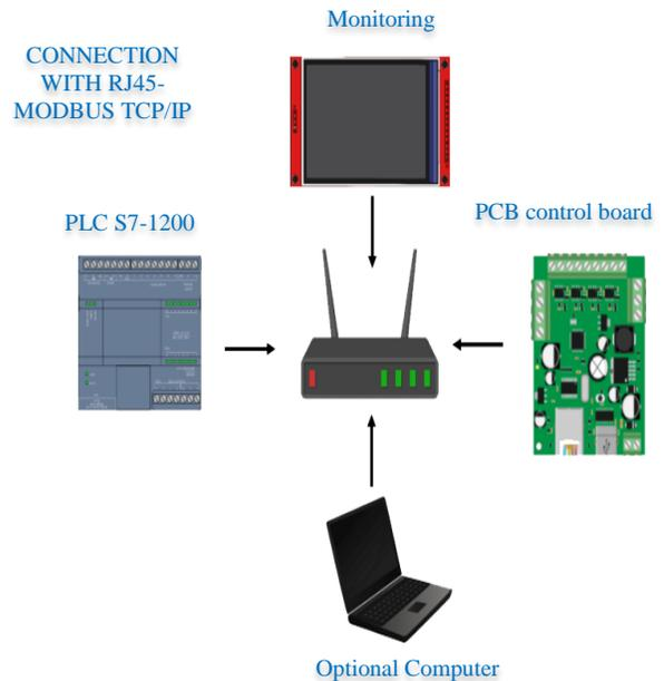
Fig. 2 MODBUS TCP/IP system
