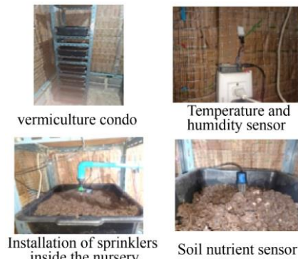
Fig. 9 Equipment of the automatic vermiculture breeding condo
