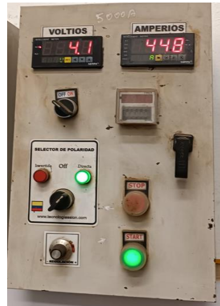
Fig. 15 SCR grinder control board
