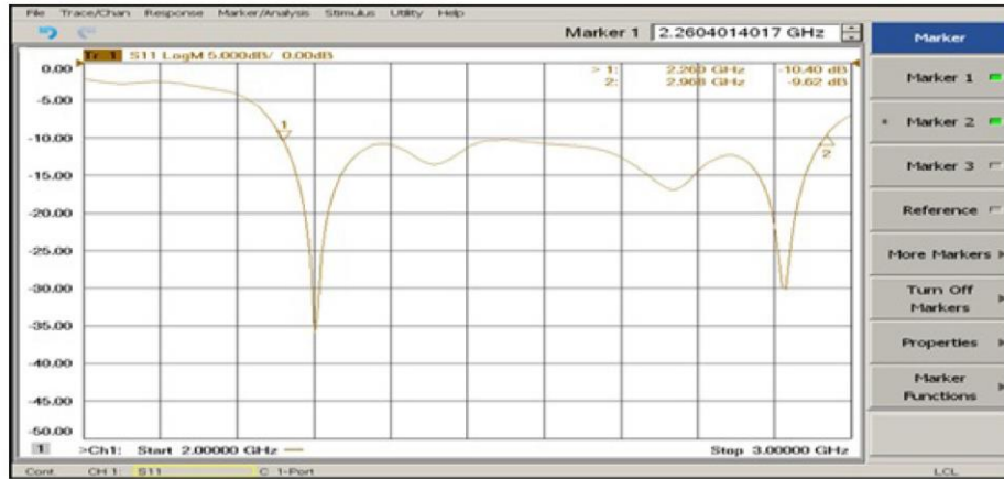
Fig. 7(a) S11 plot of simulated antenna when D1 OFF & D2 ON, and (b) S11 plot of the simulated antenna, plotted on VNA when D1 is OFF and D2 is ON.
