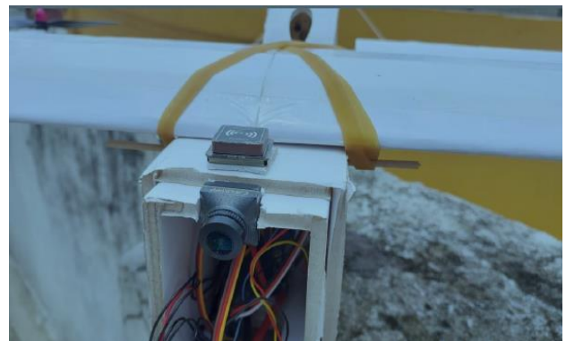
Fig. 9 FPV Camera for live video feed and GPS for navigation
