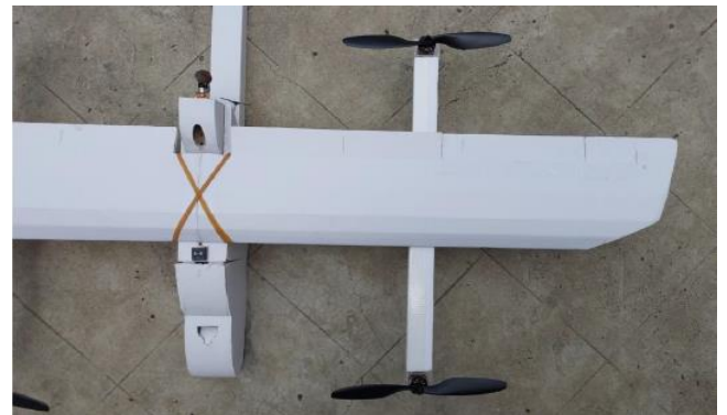
Fig. 8 Vertical lift motors for vertical take off
