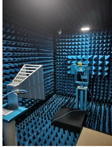
Fig. 6 Antenna gain measurement set up in Anechoic chamber
