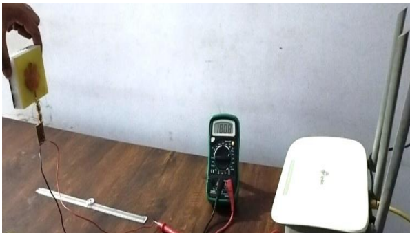
Fig. 12 Rectenna measurement Setup
