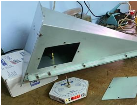
Fig. 8 Tx inside and Rx outside setup at 5 GHz
