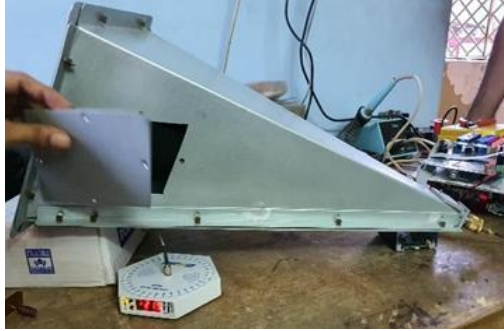
Fig. 9 Rx inside and Tx outside setup at 5GHz
