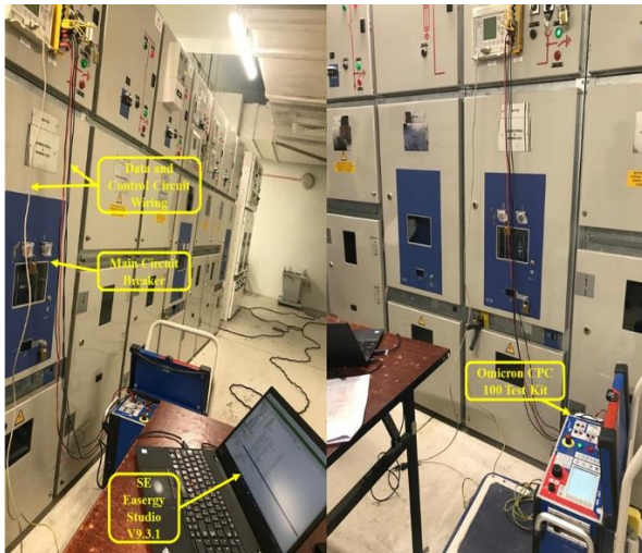
Fig. 10 Hardware In Loop (HIL) test setup
