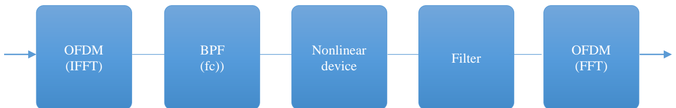
Fig. 3 OFDM model in band pass non-linearity
