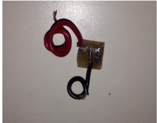
Fig. 4 Implemented biasing circuit for the diode
