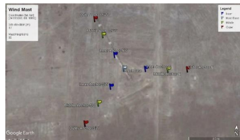
Fig. 2 Shows the wind mast with its anchors
