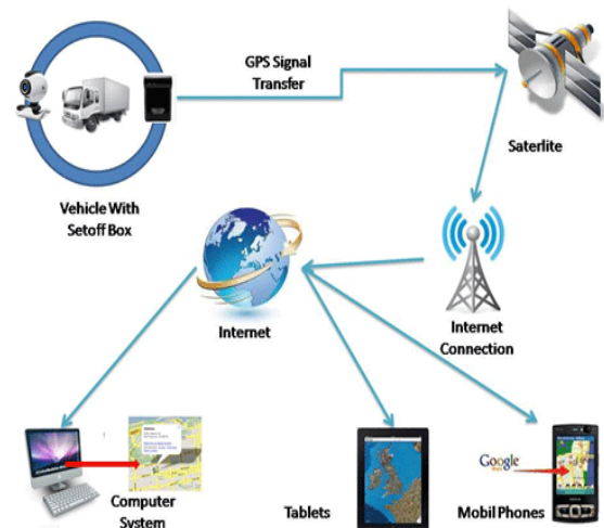
Fig.1 Operation of GPS
